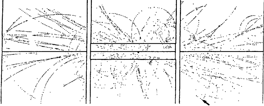
Fig. 2.8. One of the first events attributed to production and decay of a W boson, W^+ \rightarrow e^+ + \nu_e . The picture shows a reconstruction of the drift chamber signals in a large detector, UA1, surrounding the beam pipe of the CERN proton–antiproton collider. These signals originated in the collision of a 270 GeV proton (from the right) with a 270 GeV antiproton (from the left). Among the 66 tracks observed, one, shown by the arrow, is a very energetic (42 GeV) positron identified in a surrounding electromagnetic calorimeter. The transverse momentum of the positron is 26 GeV/c, while the missing transverse momentum in the whole event is 24 GeV/c, consistent with that of the neutrino (from Arnison et al. 1983).
