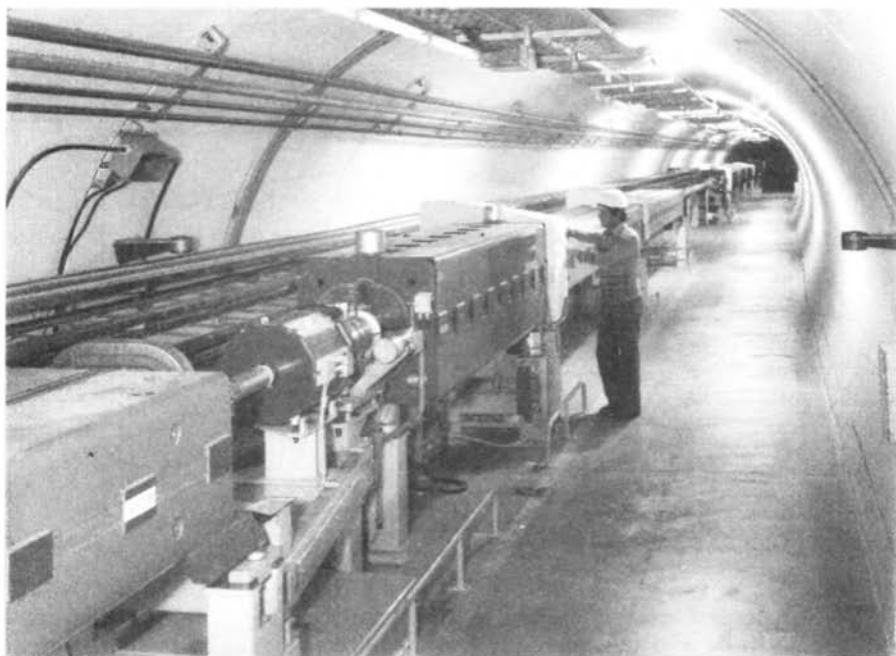
Fig. 11.4. A section of the underground 6 km tunnel of the CERN SPS machine, which accelerates protons to 450 GeV and has also been used to store and collide 300 GeV proton and antiproton beams circulating in opposite directions in the same beam pipe. The SPS also serves as an injector to the larger, 27 km circumference LEP e^+e^- ring, which in turn will also be used with superconducting magnets (Figure 11.2(c)) for the LHC pp collider.
